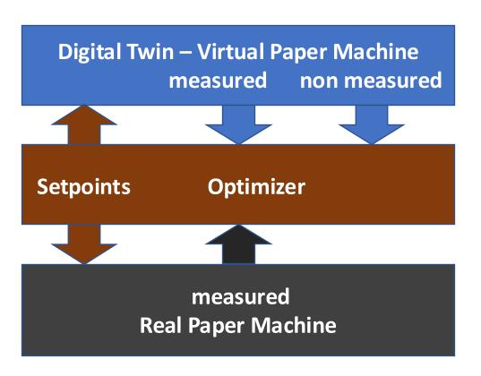
Both machines (real and virtual) are controlled with the same setpoints.
